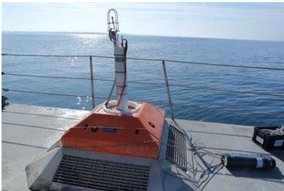
Corps mort 400 kg de type structure pyramidale de 1,7m*1,7m*1,3m
